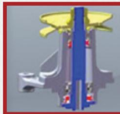
**Blade Spindle Assembly** - A forged spindle shaft for optimum strength. Die cast aluminum housing for better heat dissipation. Innovative lubrication design places each ball bearing in its own sealed compartment within the spindle housing ensuring permanent lubrication (available on 25" models).
